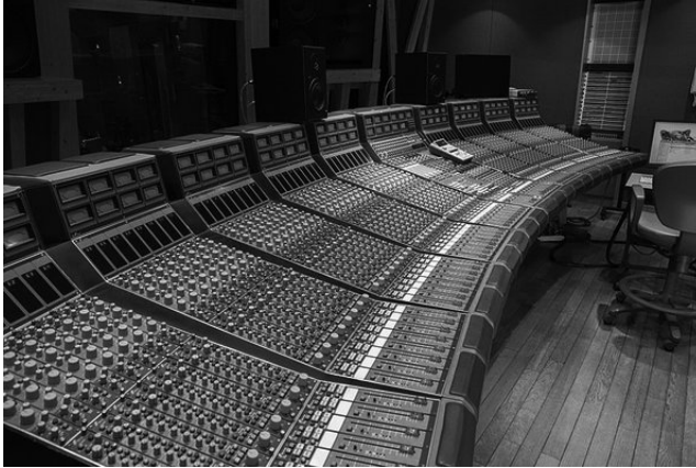
Figure 13.38. A multi-channel mixer console by Focusrite with support for 72 inputs and 48 outputs.
