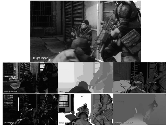
Figure 10.62. Screenshots from Killzone 2 by Guerrilla Games, showing some of the typical components of the G-buffer used in deferred rendering. The upper image shows the final rendered image. Below it, clockwise from the upper left, are the albedo (diffuse) color, depth, view-space normal, screen-space 2D motion vector (for motion blurring), specular power and specular intensity. (See Color Plate XXI.)
