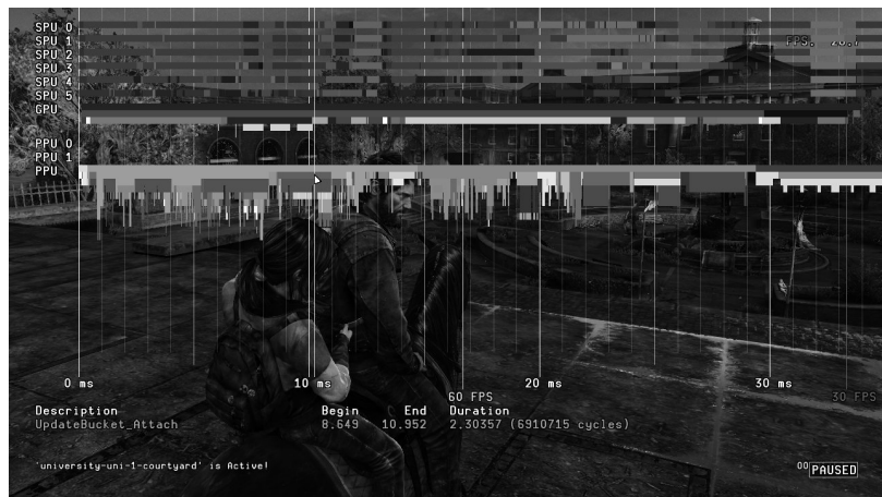
Figure 9.11. The timeline mode in Uncharted and The Last of Us (© 2014™ SCEA. Created and developed by Naughty Dog, PlayStation 3) shows exactly when various operations are performed across a single frame on the PS3's SPUs, GPU and PPU.
